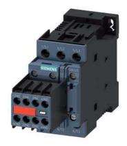
power contactor, AC-3e/AC-3, 25 A, 11 kW / 400 V, 3-pole, 24 V DC, with plugged-in diode combination, auxiliary contacts: 2 NO + 2 NC, screw terminal, size: S0, captive auxiliary switch
