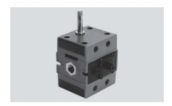
Solenoid actuated soft start valve for gradual pressure build-up in pneumatic systems. This ensures safe start-up of pneumatic systems. A minimal amount of air flows into the system via an adjustable flow control valve. Output pressure is built up slowly. Downstream cylinders and working devices are slowly advanced to their initial positions. When the
