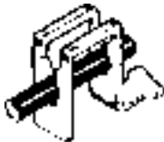
Insulation displacement connectors (IDC)
