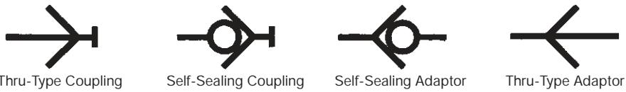
Self-Sealing Coupling and Self-Sealing Adaptor = sealing on both sides.
